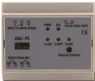
DALI BUS Power Supply : Supply power for DALI BUS..
